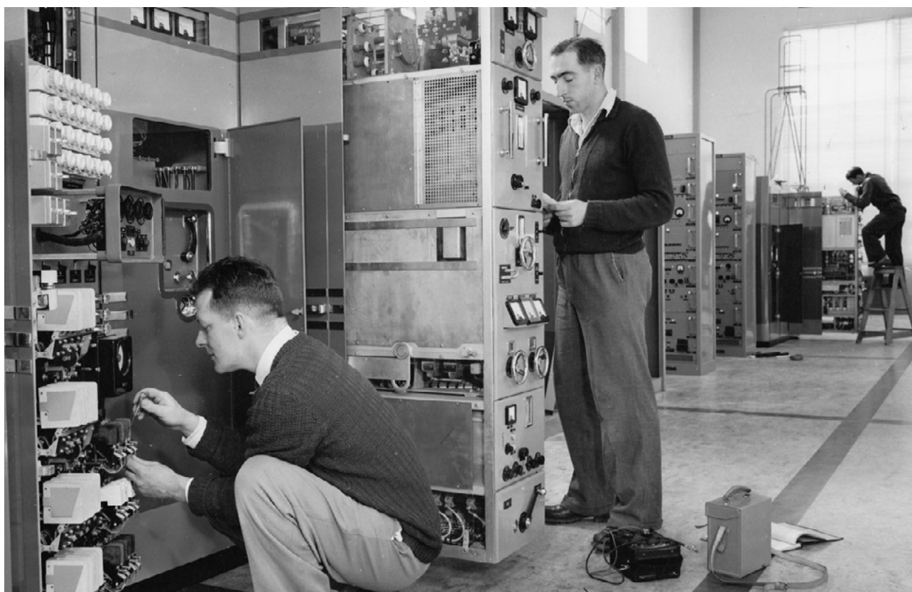
STC DS 12 Transmitters - (This type was a 4-Bay as it had a Modulator Cabinet)
